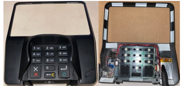
Pictured: Real skimmer removed from payment device
